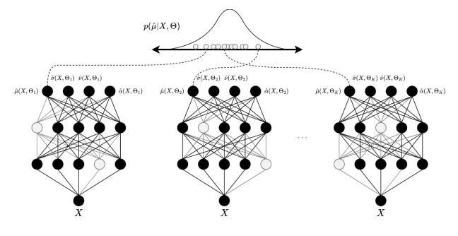
Figure 7: Bayesian Inference with MC Dropout
