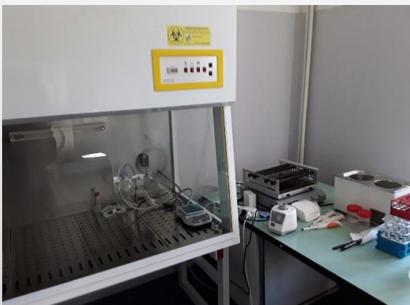
BSL-2+ wastewater processing room
