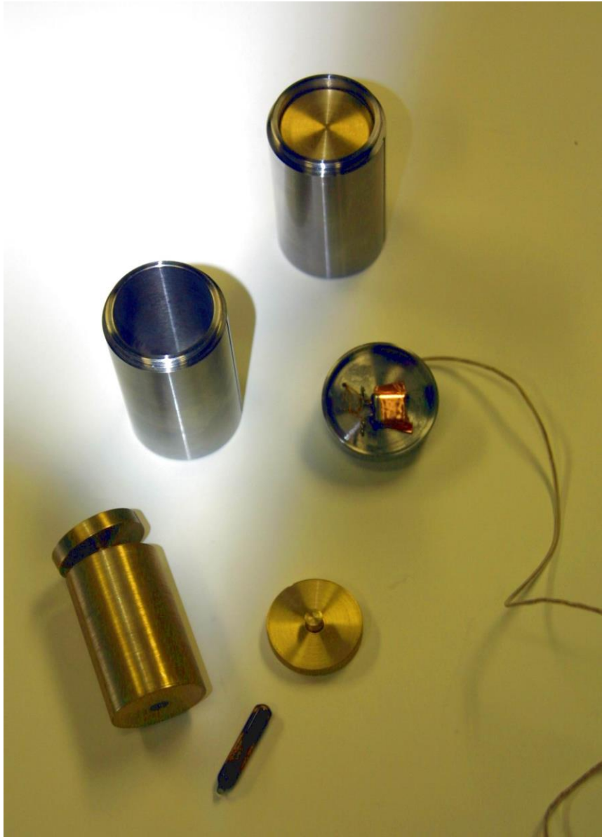
port assemblies -- source (absorbers) holders & cells
