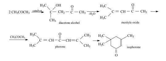
Other by-products are mesitylene, isoxylitones, tetramethyltetralone. The conversion of acetone increases with rise in temperature – from 87.4 wt% at 120° to 97.5 wt% at 370 °C.
