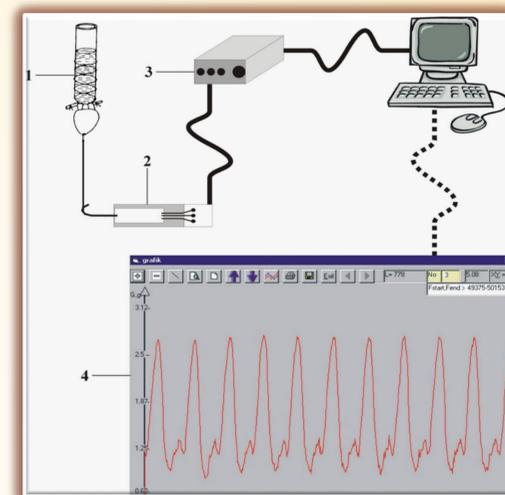
Fig.1 Experimental setup for recording of cardiac contractions TENZO-1 (Stocks, Sofia, Bulgaria). 1 - cannula with excised frog heart; 2 - force transducer; 3 - analog-digital converter; 4 - original record.
