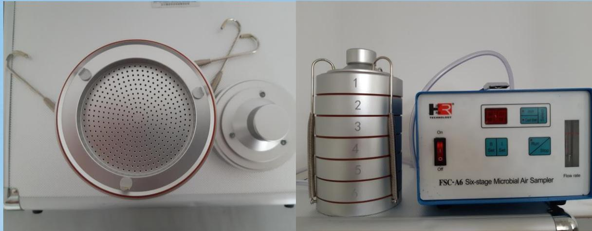
**Fig. 1.** Six-stage cascade impactor
