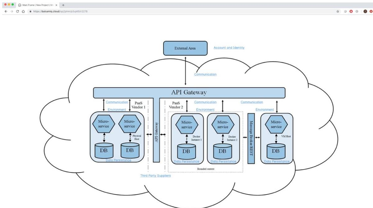
Figure 15 Scheme of a software application applying microservice architecture
