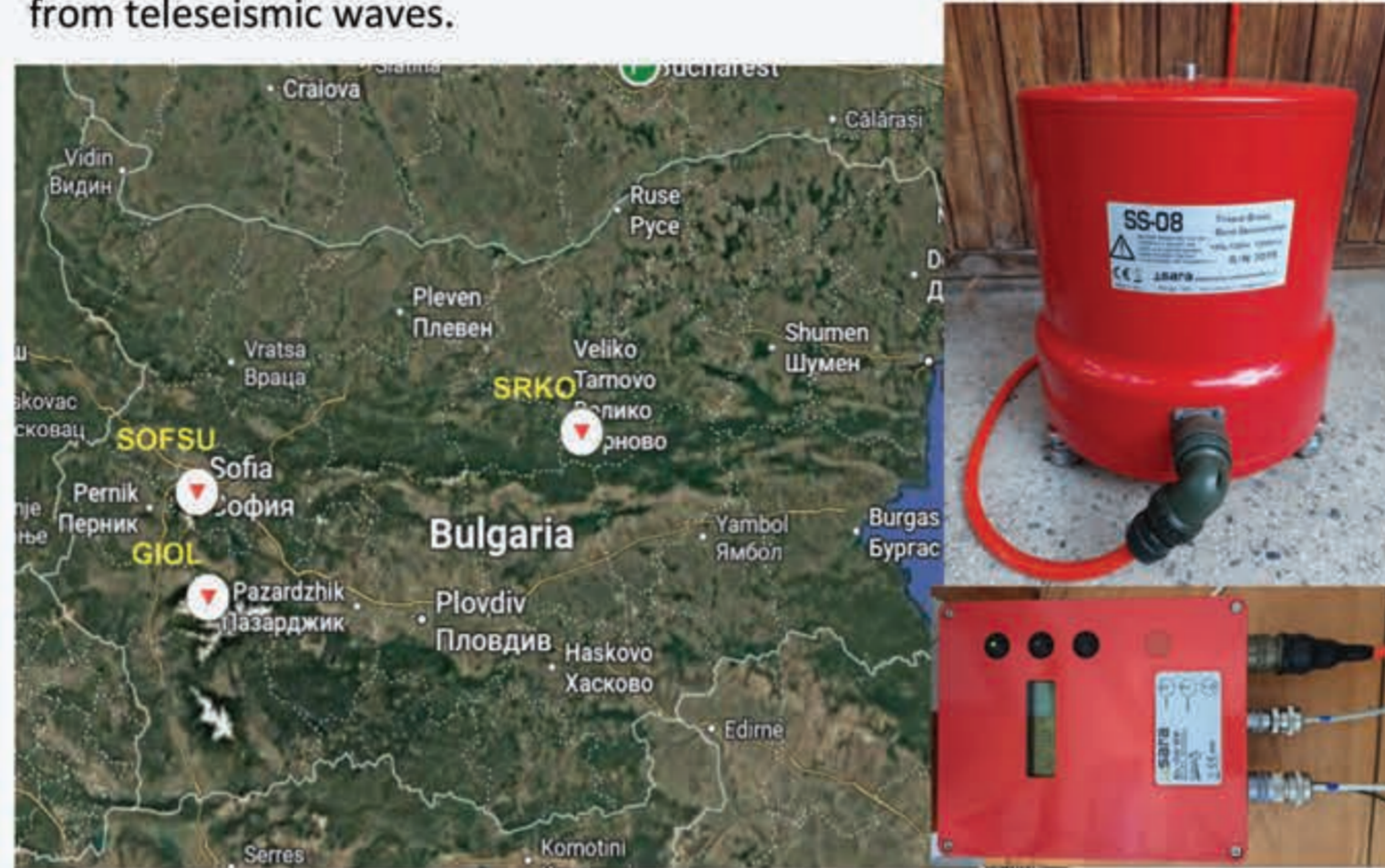
Location of the broad-band seismic stations SRKO (Sredni Kolibi) and GIOL (Giolechitza) and single-station equipment (seismometer and digitizer form SARA Electronic Instruments).
