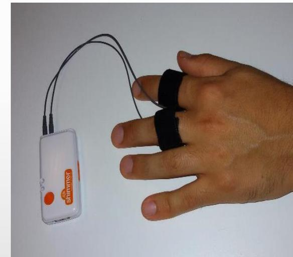
Shimmer3 GSR+ device (with a sampling rate of 128Hz) for electrodermal activity assessment
