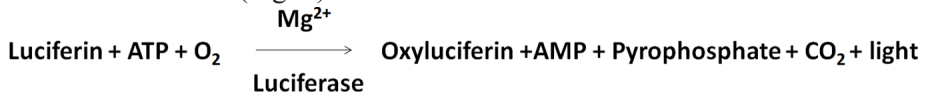
Figure 2. Quantitative ATP determination by using a recombinant firefly luciferase and its substrate D- luciferin. The assay is based on a simple luciferase assay, which requires ATP for the enzymatic reaction to produce luminescent light (emission maximum is approximately 560 nm at pH 7.8).
